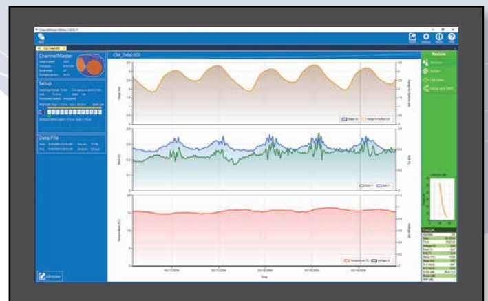
Above: ChannelMaster H-ADCP data sample. Below: The ChannelMaster H-ADCP is installed on a riverbank or near-shore structure to acquire real-time velocity, stage, and discharge data.
